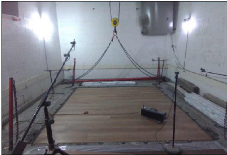
Photo No. 1 Source Room View of Test Specimen Installation
