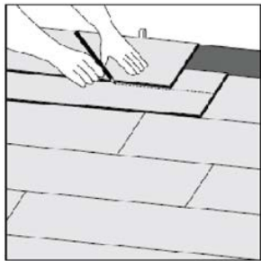
Step 6 Measure and cut final row of planks allowing for 5 mm expansion gap
